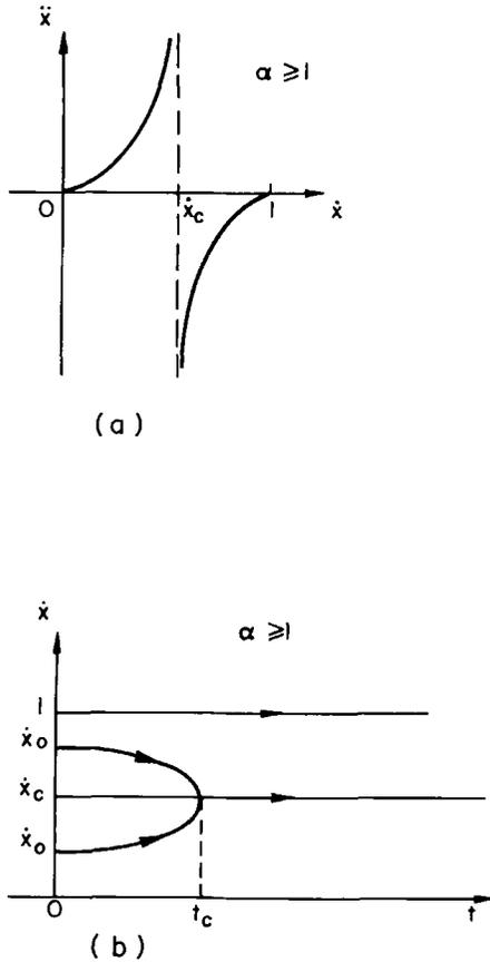
Fig. 2. (a) Behavior of Eq. (8) for  $\alpha \geq 1$ . The acceleration goes to infinity when the velocity tends to the critical velocity,  $\dot{x}_c$ , given by Eq. (10). For  $\alpha = 1$  the critical velocity is zero,  $\dot{x}_c = 0$ . (b) Situation for  $\alpha \geq 1$ .
